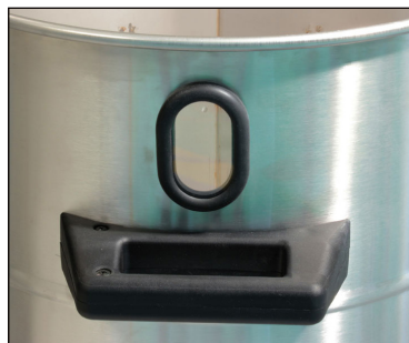
Sight glass installed on recovery tank
